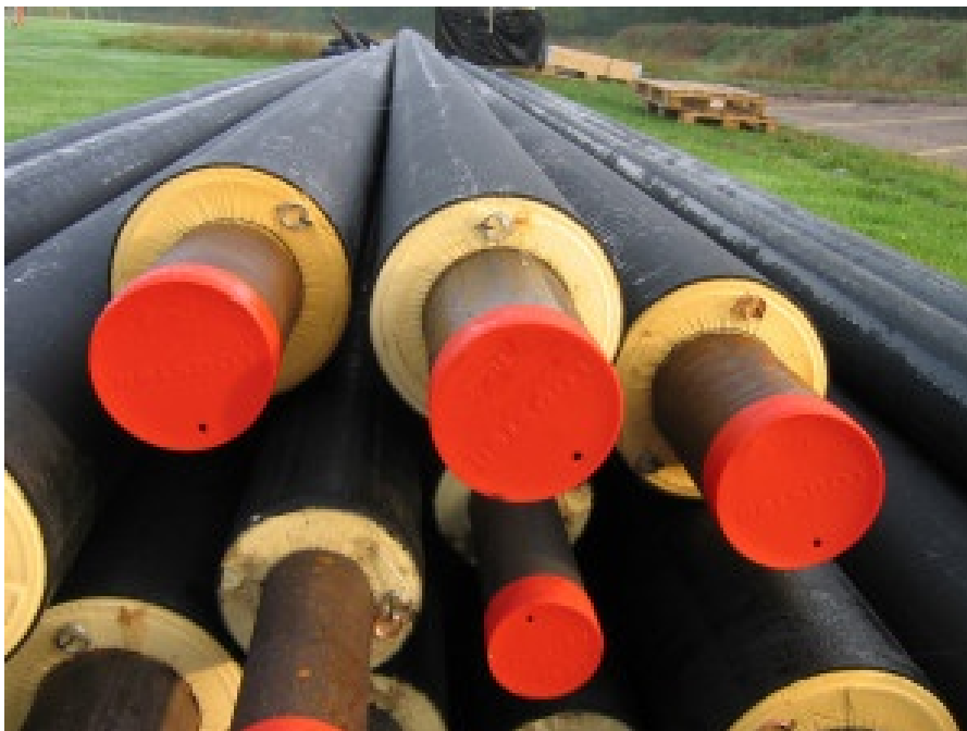
Figure 2 Photograph of typical DH pipes
